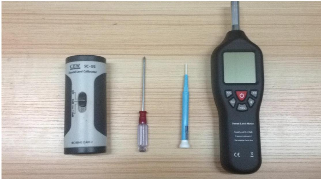
Step 1: Use the Metal screwdriver to open the back cover of the meter.
